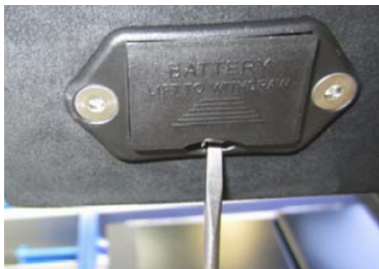
用平口螺丝刀打开电池箱盖
